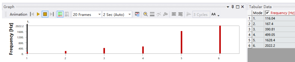
Figure 26 Medium mesh frequency analysis
