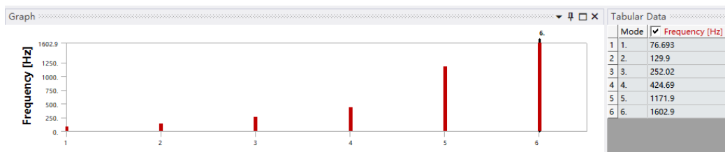
Figure 11 natural frequency for coarse mesh size
