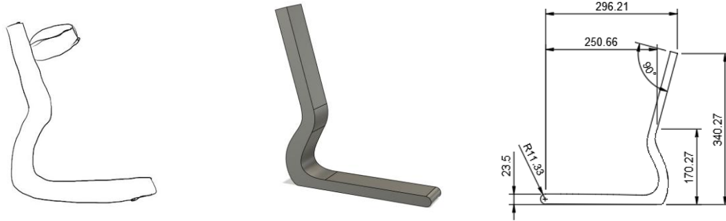
Figure 4 Initial sketch and corresponding CAD model of the baseline running blade design
